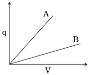
The given graph shows variation of charge 'q' versus potential difference 'V' for two capacitors  $C_1$  and  $C_2$ . Both the capacitors have same plate separation but plate area of  $C_2$  is greater than that of  $C_1$ . Which line (A or B) corresponds to  $C_1$  and why?
