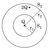
A sphere  $S_1$  of radius  $r_1$  encloses a net charge Q. If there is another concentric sphere  $S_2$  of radius  $r_2$  ( $r_2 > r_1$ ) enclosing charge 2Q, find the ratio of the electric flux through  $S_1$  and  $S_2$ . How will the electric flux through sphere  $S_1$  change if a medium of dielectric constant K is introduced in the space inside  $S_2$  in place of air?
