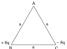
Two point charges + 6q and - 8q are placed at the vertices 'B' and 'C' of an equilateral triangle ABC of side 'a' as given in the figure. Obtain the expression for (i) the magnitude and (ii) the direction of the resultant electric field at the vertex A due to these two charges.
